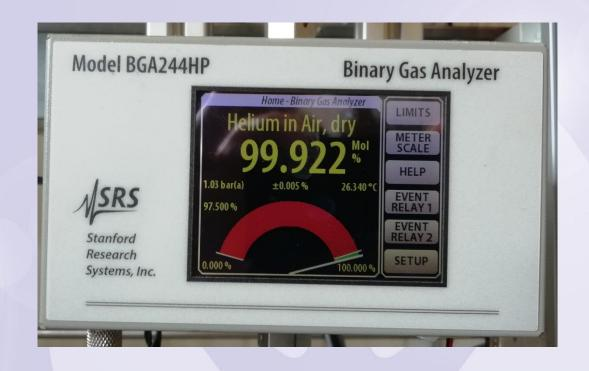
Two common methods, thermal conductivity of gas or speed of sound principle! diamond
