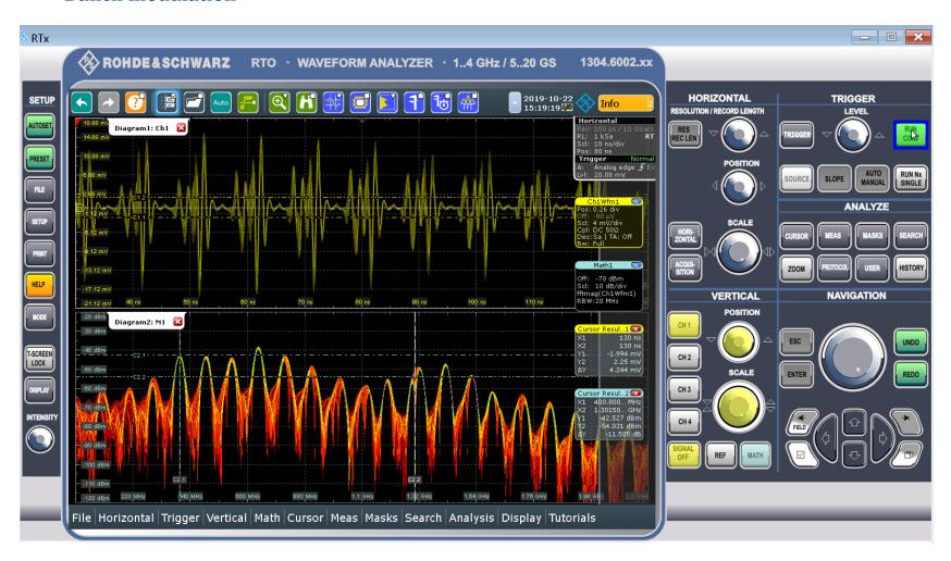
Filling pattern measured on striplines show 800MHz-1,3GHz modulation of individual bunches
