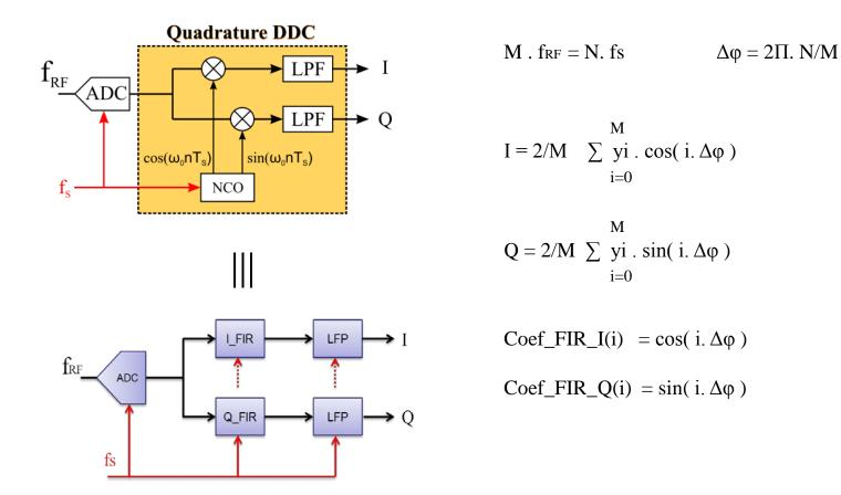
By down-sampling a RF signal, we can calculate precisely I and Q. But we need few RF period instead of one with a classical IQ demodulation.
