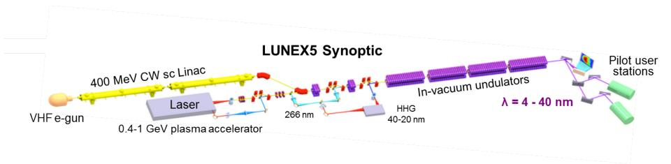
Phase 1 : based on a 400 MeV CW sc Linac → explore advanced FEL techniques and applications Phase 2 : laser wakefield (or plasma) accelerator will be assessed in view of FEL applications
