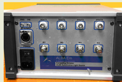
Image of the electrometer developed at ALBA. Photograph: ALBA
