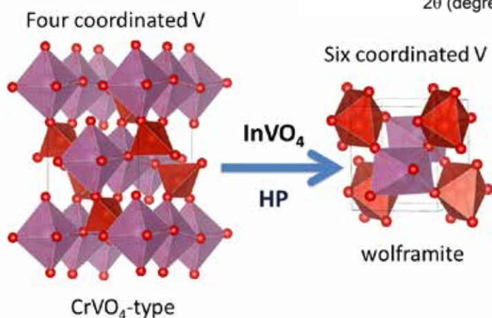
Fig. 12: Crystal structure of the low- (left) and high-pressure (right) phases. The coordination change of V can be clearly seen in the figure.
