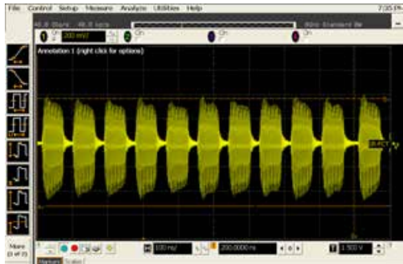
Figure 29: FCT image of the beam filling pattern at the SR.
