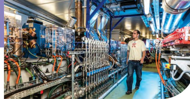
The accelerated electrons, when passing through magnetic fields, bend their trajectory and emit **synchrotron light**, which reaches the beamlines (laboratories).
