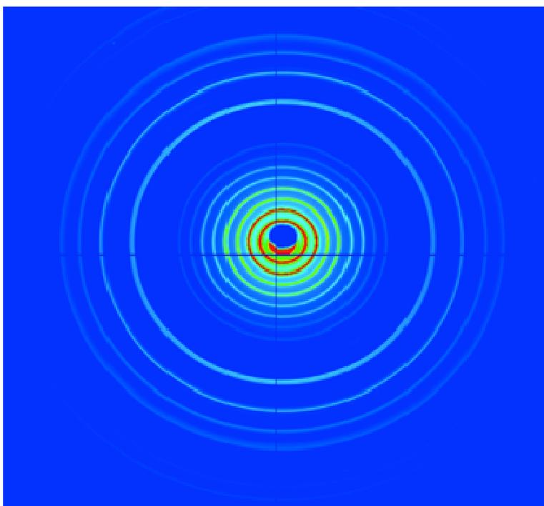
**Figure 1. BL11-NCD:** A 1 second exposure of silver behenate collected on an ADSC210 CCD detector with a sample to detector distance of ca. 220 mm is illustrated.
