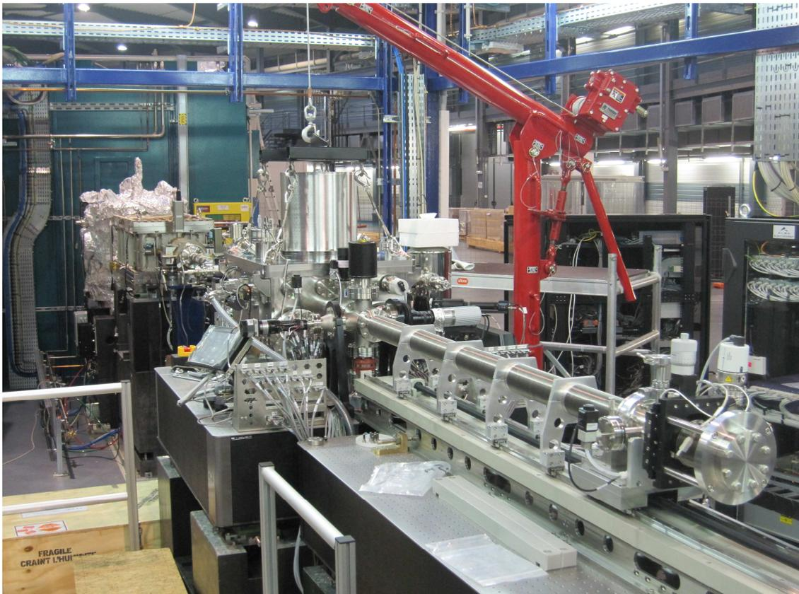
**Figure 1.** Beamline 09 (MISTRAL) with the recently installed transmission X-ray microscope.
