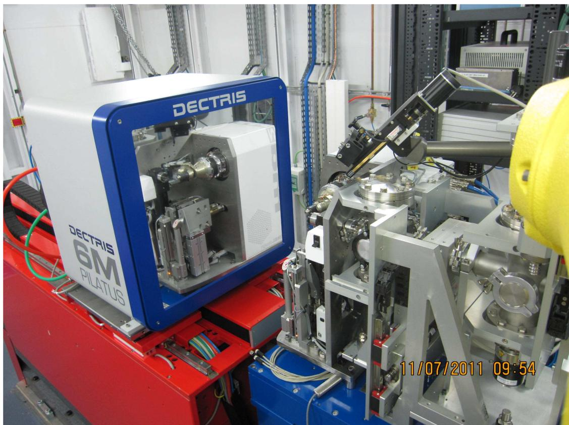
**Figure 3. BL13-XALOC:** The PILATUS 6M detector installed at the beamline.
