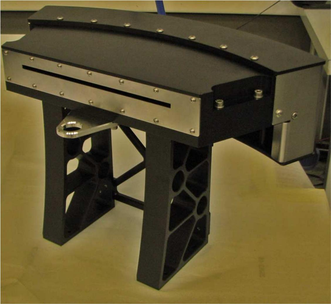
**Figure 1.** The fast position sensitive strip-detector (SLS Mythen 2 design) of BL04-MSPD.
