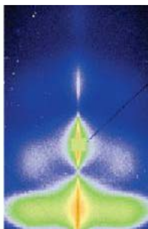
Fig.10 \mu\text{GISAXS} pattern of a self-assembled nanometer-sized gold cluster layer on top of thin polymer layer on a silicon substrate [10].
