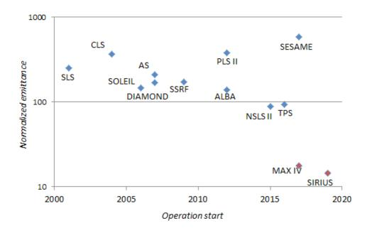
Figure 8 – Emittance normalized with circumference and square of energy plotted versus year of operation start of light sources included in Table 4. Blue dots correspond to 3rd generation light sources, red to 4th ones.
