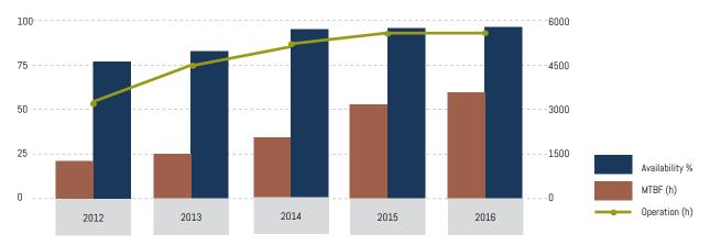
Figure 5- Operation summary. Availability (in %) and MTBF (in h) are on the left vertical axis. Operation hours per year on the right one
