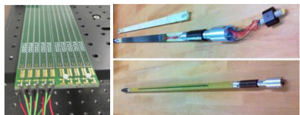
Figure 40: Multilayered PCB with radial coils developed at ALBA outside and inside the shaft used for carrying out integral measurements of multipole magnets.
